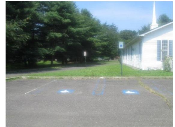
Parking spaces can be replaced with porous asphalt to capture runoff from the road and roof. A rain garden can also be planted along the side of the building to capture, treat and infiltrate rooftop runoff. A preliminary soil assessment suggests that soils have suitable drainage characteristics for green infrastructure.
