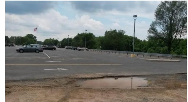
Stormwater drains to an existing detention basin near the entrance of the school. Pervious pavement can be used to infiltrate parking lot runoff. Downspouts in the back are already disconnected and can be directed into rain gardens and planter boxes to capture, treat and infiltrate runoff. A preliminary soil assessment suggests that the soils have suitable drainage characteristics for green infrastructure.
